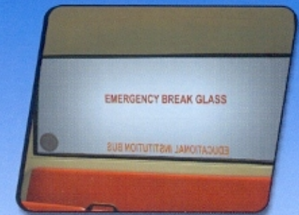
Large emergency exit window
