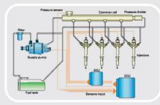
Common Rail Diesel Engine Technology (CRDe) ensures fuel is always stored and injected at a high pressure
